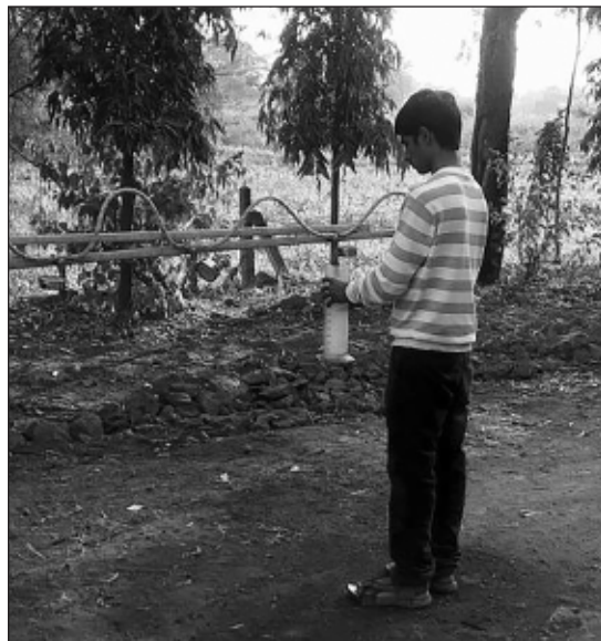
Fig. 7. Set-up for pressure and discharge measurement of nozzles
