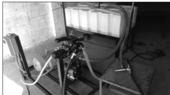
Fig. 4. Pressre relief valve testing set-up
