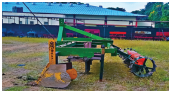
Fig. 1. Light weight multi crop basin lister seeder.
